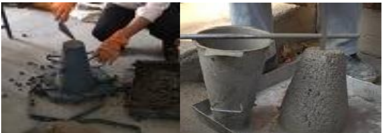
Fig 4: Slump Flow Test
