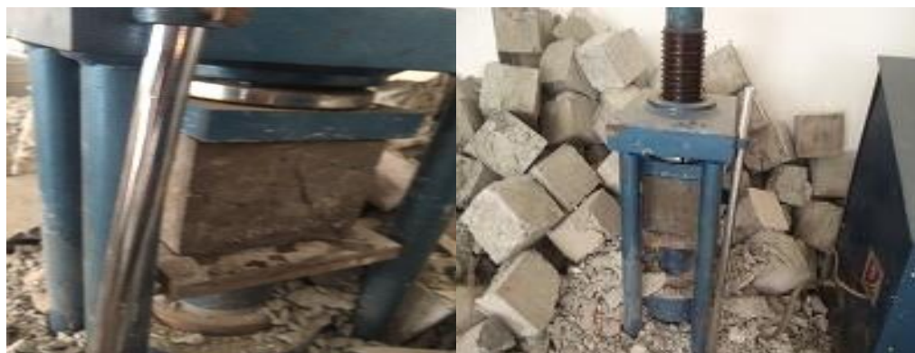
Fig 6: Checking of Compressive Strength
